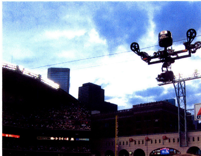
Figure 2: Skycam cable robot at a baseball stadium [26].
