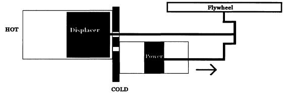
**II. Transfer of Air from the Hot Side to the Cold Side:** This is the second step in the Stirling Cycle. When the power piston moves outward during the expansion step, the links that connect the two pistons cause the displace piston to move to the left. If the displacer piston moves to the left, the air has to squeeze around it and move to the right. So the air goes from the hot side of the engine where the flame is to the cold side of the engine away from the flame.
