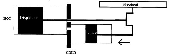
**IV. Transfer of Air from the Cold Side to the Hot Side:** This is the fourth and final step of the Stirling Cycle. When the power piston moves back inward to the left, the links that
