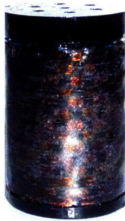
Figure 18: Finished carbon fiber and copper co-wound Lorentz force coil
