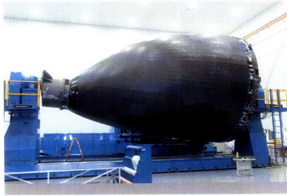
Figure 3: Nose part of a Boeing 787 Dreamliner composed of a single composite part before doors and windows have been cut. Reproduced from [10].
