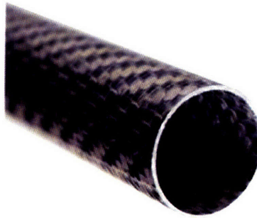
Figure 2: Carbon fiber tubing. This configuration is generally created from dry lay-up or resin induction. Reproduced from [9].
