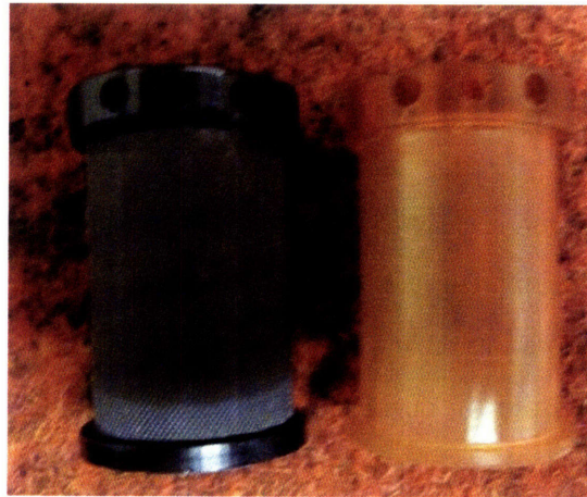
Figure 15: Comparison of carbon fiber and plastic bobbin. The carbon fiber bobbin (left) that is created by wet lay-up has similar dimensions as the plastic bobbin (right) created on a CNC lathe.
