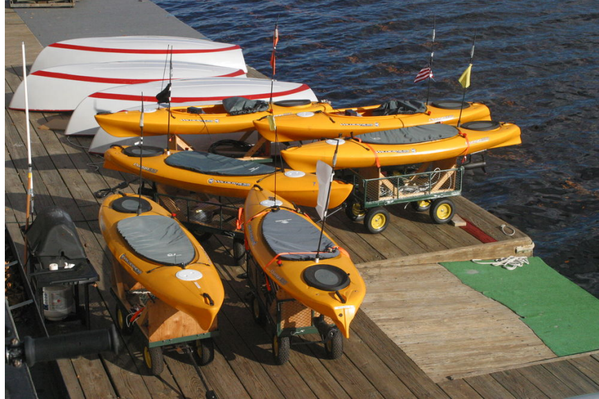
Figure 1-4: The SCOUT platform of autonomous kayaks are a relatively inexpensive robotic platform. The low cost and ease-of-use make it possible for research groups to own and operate several of these vehicles. Image courtesy Mike Benjamin.
