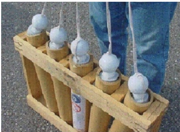
Fig. 5. Inserting bombs into a shot tubes mortar battery in fan.
