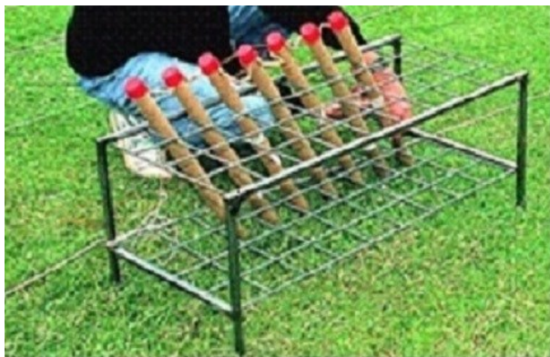
Fig. 4. Mounting an inclined battery by roman candles.
