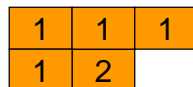
Figure 5. Macroblock dependence in image processing section of H.264. A macroblock is dependent on neighboring macroblocks above-left, above, above-right, and to the left. All macroblocks labeled “1” must be processed before the macroblock labeled “2.”
