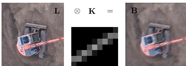
Figure 3: Visual illustration of the blur convolution. At the left the original or pure image ( \mathbf{L} ), is convoluted with the blur kernel ( \mathbf{K} ). Here the brightness intensity of this matrix is related to value intensity, where the brightest value corresponds to 0.1. The result of the convolution ( \mathbf{B} ) is illustrated on the right.
