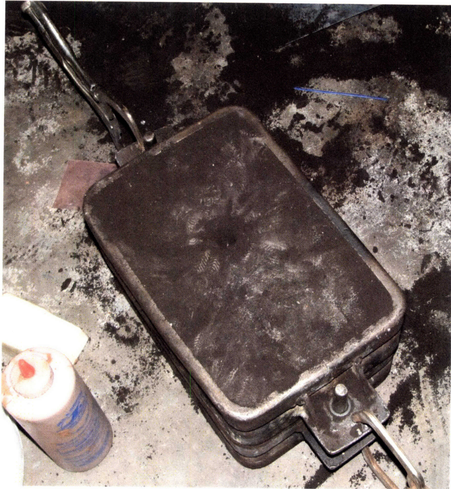
Figure 5: This photograph shows a packed mold mated, clamped, and awaiting molten metal. Note the chassis pattern and mold adhesive in the bottom right.
