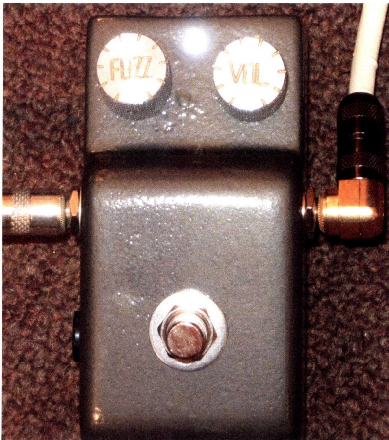
Figure 19: The completed guitar effect pedal being tested. Note the lit white LED indicating the effect is engaged.
