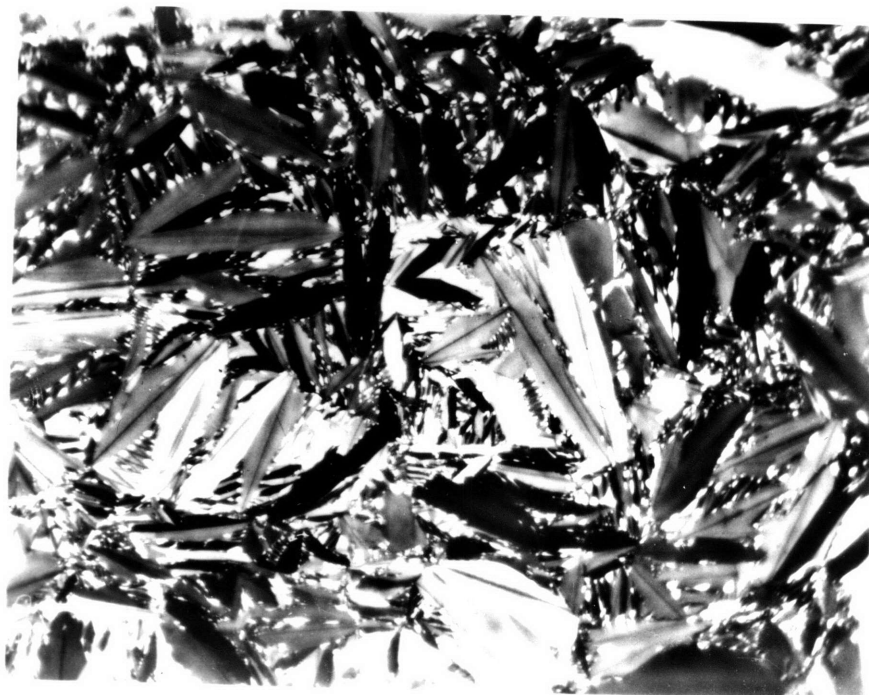
FIG. 21 ZERO - FIELD BURSTING MORPHOLOGY IN Fe 30.8 Ni
