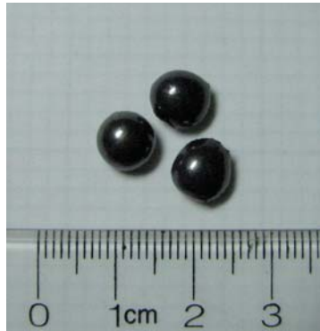
Fig. 10-6. Photograph of Ce shot used for electron beam deposition.
