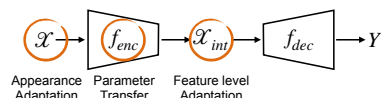
Figure 4. Parts of an abstract deep learning model f affected by different kinds of domain adaptation
