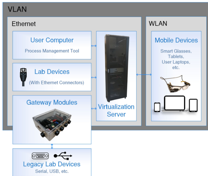
FIGURE 1 Overview of the hardware used in the digitized laboratory. All components are connected to the same VLAN (Virtual Local Area Network) either with wire-based Ethernet connections or to WLAN. Legacy devices are connected to the network using hardware gateway modules. With this network architecture, the flawless communication of all devices is ensured
