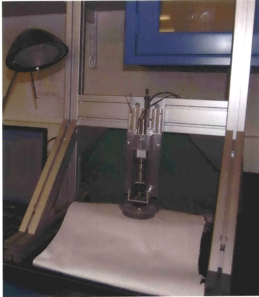
Figure 3-9: Frame for mounting tool in the laboratory
