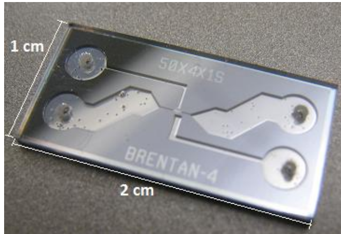
Figure 30: Image of a device after dicing and separation from the wafer.
