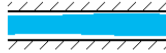
Figure 40: Hydrophobic walls in a channel produce an annular flow, with gas hugging the walls and liquid trapped in the center.
