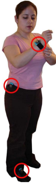
Figure 5-43: Placement of the three wireless accelerometers during the real-time evaluation experiment. The sensors were worn at the hip, dominant wrist, and dominant foot, right on top of the shoe laces.
