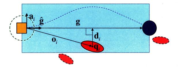
Figure 4-7: Collision corridor with two obstacles outside the corridor ignored (dashed ellipses). The green dashed circle around the orange vehicle square is the critical range used to initiate emergency reverse maneuvers. The corridor is a three-dimensional cylinder, flattened in these diagrams to facilitate discussion.
