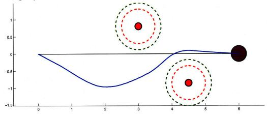
Figure 4-11: A little more unusual arrangement with staggered obstacles. Because the vehicle places higher weight on obstacles with sooner time to impact, it avoids the nearer obstacle first, slaloming between them.
