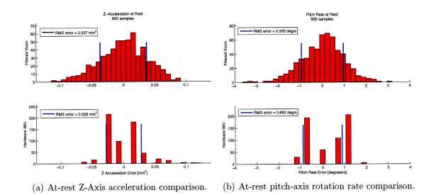
Figure 2-7: At-rest inertial data comparison.
