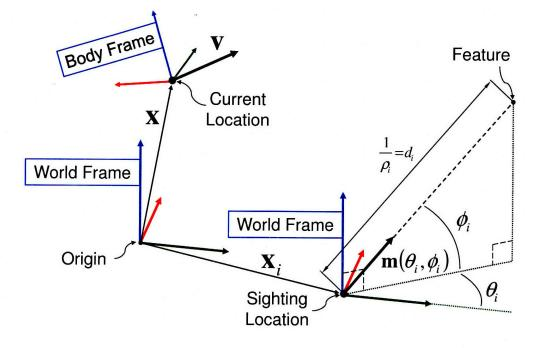
Figure 3-4: Position and velocity are represented in the world frame from the origin. Feature azimuth and elevation bearing angles are measured in the world frame from  $\mathbf{x}_i$ , the point of first sighting.  $R^{WB}$  defines the body frame.
