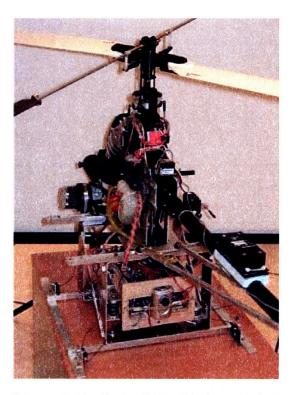
Figure 1-6: A typical vision-equipped autonomous helicopter [8].
