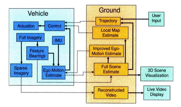
Figure 1-10: System architecture.
