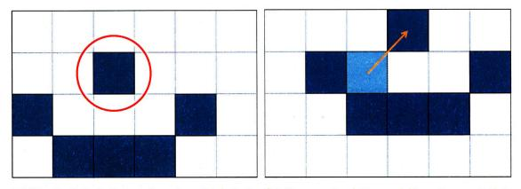
(a) Identical pixels form a shape based on relative (b) Context shows the same shape is repeated, incontext. Red circle indicates pixel to track. dicating the tracked pixel has moved up and right.
