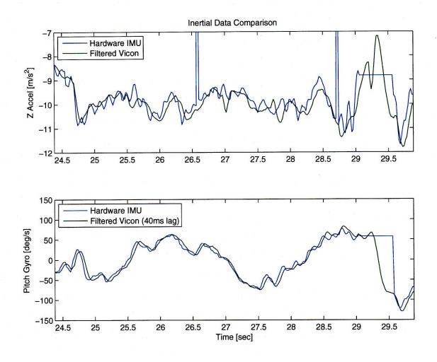
Figure 2-6: Comparison between inertial data measurement systems. Note dropout between 29 and 29.5 seconds.
