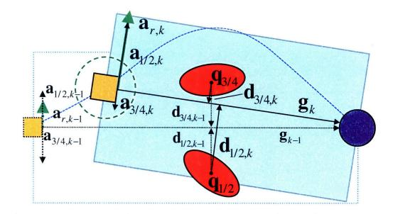
Figure 4-8: Top view of potential obstacle "net" situation. At time k - 1 the effects of the obstacles almost perfectly cancel, but the vehicle still reacts intelligently.
