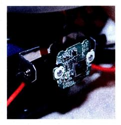
Figure 2-4: Closeup of camera with mount and ribbon visible.
