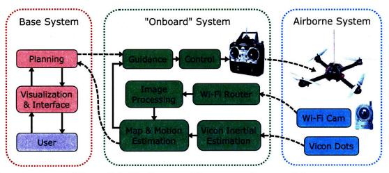
Figure 2-1: Hardware architecture and connectivity.
