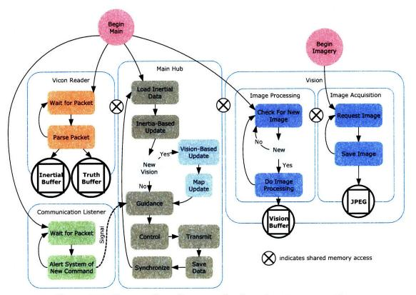
Figure 2-8: Process flow diagram of onboard system operation.
