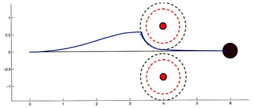
Figure 4-10: A very unusual scenario with a symmetric obstacle "net". The vehicle gets a little confused, but ultimately finds the gap between the obstacles using the emergency avoidance routine.
