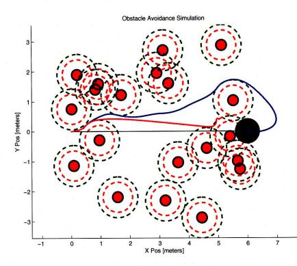
Figure 4-12: A comparison of repulsion only trajectory in magenta vs. the corridor augmented technique in blue with 20 obstacles in the plane z = 0.
