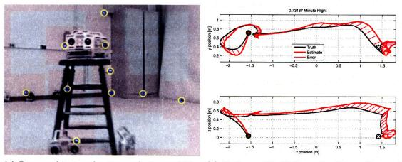
(a) Processed image showing occlusion and blur- (b) Orthographic flight path plots. Green cirring.
