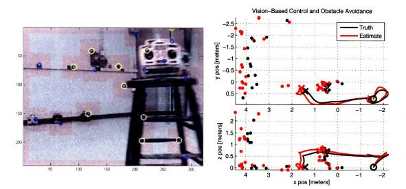
(a) The circles indicate points being tracked yellow for ego-motion estimate filter, blue for mapping.
