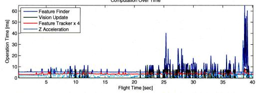
Figure 5-11: Processing time of finding and tracking features, conducting vision updates, and current Z acceleration as the flight progressed.
