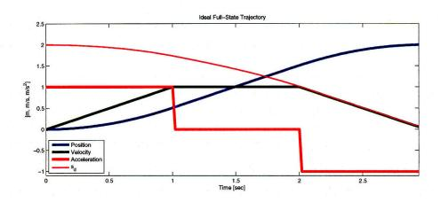
Figure 4-2: An ideal movement trajectory simulated in one dimension.
