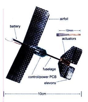
Figure 1-5: UC Berkeley 2 gram autonomous glider [68].
