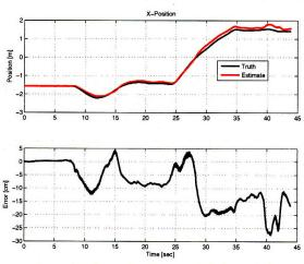
(d) X-axis position estimate error propagation during the flight.
