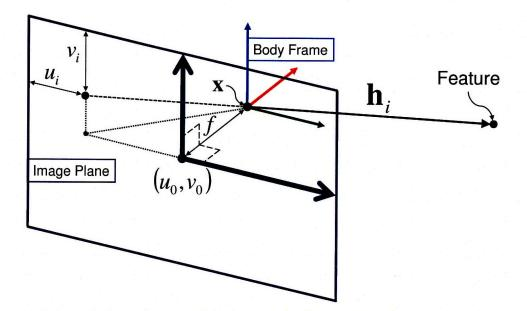
Figure 3-5: Pinhole camera model showing (u, v) pixel coordinates of a tracked feature. The purple box is the image plane, f is the camera focal length, and  $\mathbf{h}_i$  is the body-frame vector from the current vehicle position to the tracked feature.
