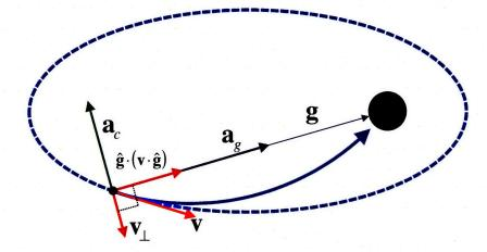
Figure 4-3: Acceleration components toward the goal and perpendicular to the goal vector combine to fly the vehicle directly into the goal.
