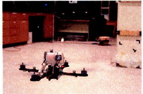
Figure 2-2: Closeup of quadrotor with Figure 2-3: The quadrotor with camera and radios in flight. Flight computers and operator station in background.
