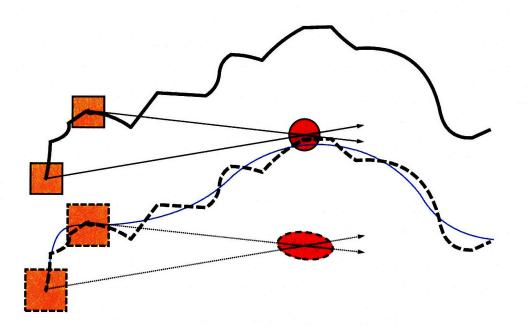
Figure 3-14: The red obstacle only needs to be mapped in a relative sense for the vehicle to avoid it.
