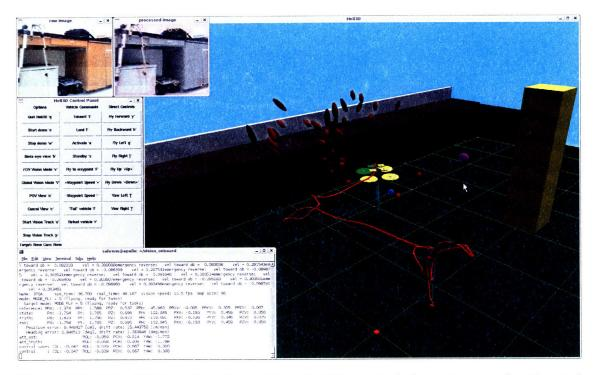
Figure 2-9: The 3D interface for point-and-click control shows true and estimated position, mapping, and control reference. Real-time vision and terminal output are also displayed.
