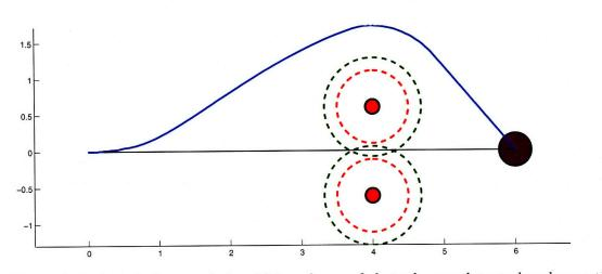
Figure 4-9: A typical scenario in which a clump of obstacles are detected and smoothly avoided. A typical potential function solution would get stuck in the notch between the obstacles.
