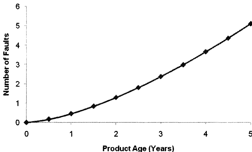
Figure 4-3: Expected number of faults over product age when d = 0.6 , k = 1.5 , and \lambda = 1
