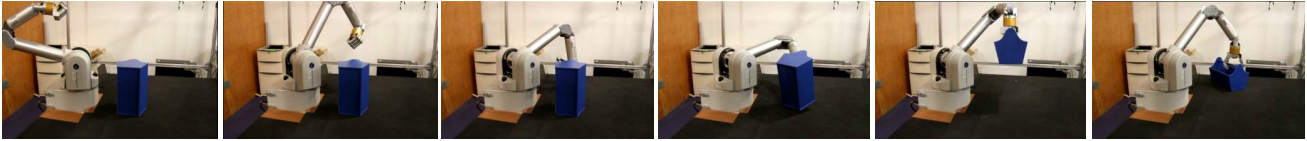
Figure 9. Some snapshots taken in the process (from left to right) of our robot's grasp of a basket.
