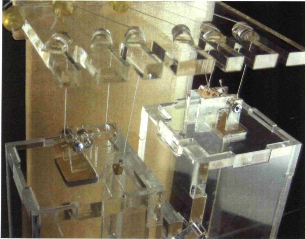
Figure 30: Rounded bearing surfaces guide the cables through the last turn downward to the actuating lever arm
