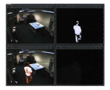
Figure 4-5: Output of the program run in the example. (upper left) the current background image. (lower left) the current frame. (upper right) the connected component which remained after filtering. (lower right) the current depth map in a very early stage of development. As the depth map is refined, it nears the approximate depth of the scene.
