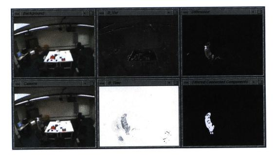
Figure 4-4: (left column) The current background and the current image. (middle column) The variance and frequency for the model of each pixel in the background. Lighter pixels in the variance image correspond to pixels which vary more. Lighter pixels in the frequency image correspond to pixels which have more consistently occurred in the recent past. (right column) The binary image of pixels which are not part of the background and the filtered connected components.
