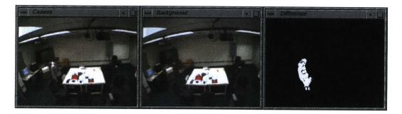
Figure 3-1: An example of backgrounding showing (left) the current frame, (middle) the background, and (right) the thresholded difference between the background and current frame giving the pixels which are significantly different from the background. The human figure which is not part of the background is visible in the difference.
