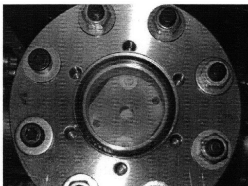
Figure 2.23: Sample and sample holder as seen through the window of the vacuum chamber.
