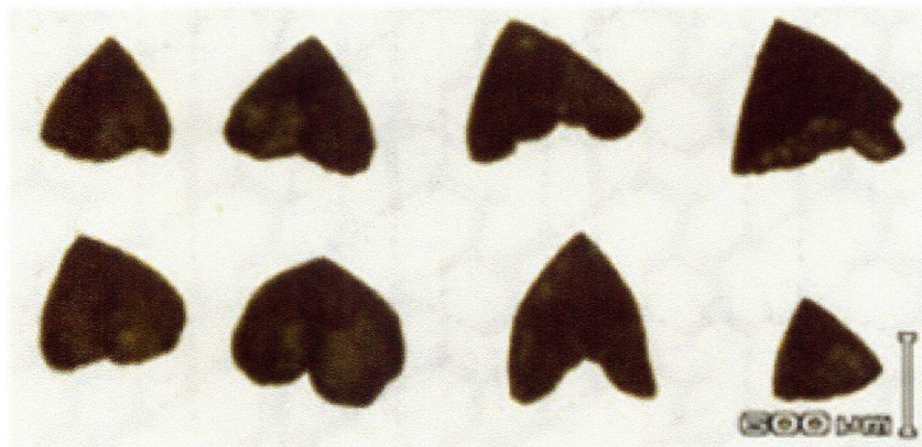
Figure 3-6: \gamma -glycine crystals observed in several crystallizations from a 1:1 water-ethanol solution.[4]
