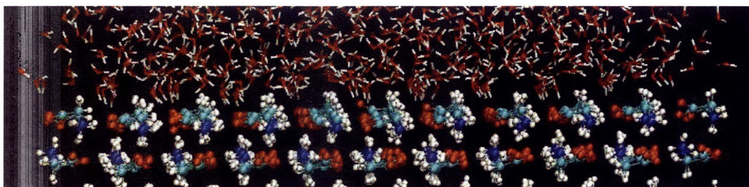
Figure 5-10: Schematic of the interface with water and (010) face of \alpha -glycine with C—H groups exposed.
