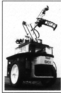
Figure 6-2: Our mobile manipulator with a two link arm and gripper.
