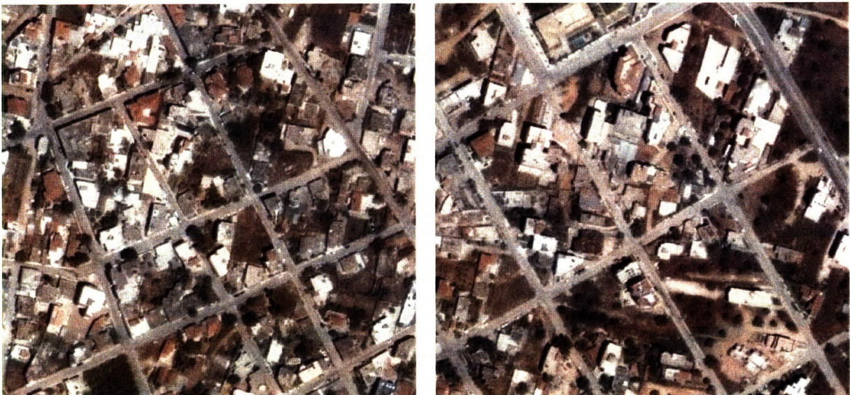
Figure 8 Grid road systems imposed on the existing agricultural subdivision- Koropi, Spata, 2008 The resulting urban form is a hybrid between the two systems with buildings following the agricultural system in size and directionality.
