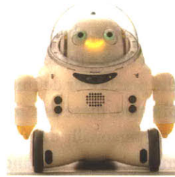
Top Fig. 2.12 Ifbot, developed by Business Design laboratory Co for elderly people, is currently on the market in Japan. Ifbot is able to respond to verbal commands and enter into dialogue.
