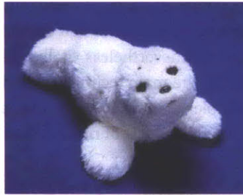
Fig. 2.13 Paro the robotic seal developed as a therapeutic robot by Takanori Shibata. Paro has sensors under its fur and can respond to human touch by changing its sounds and movements.
