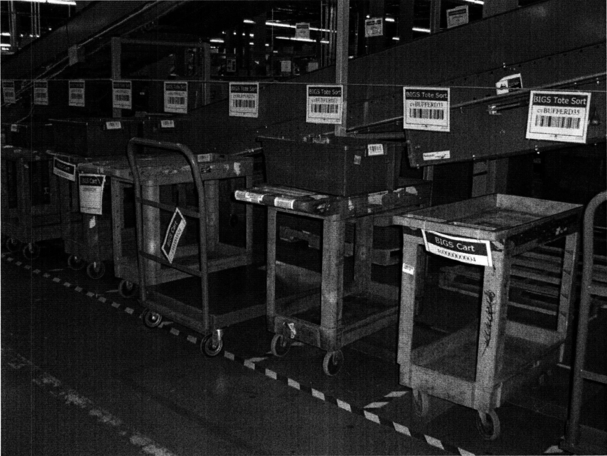
Figure 25: Tote Sortation Area showing buffer locations, carts and totes
