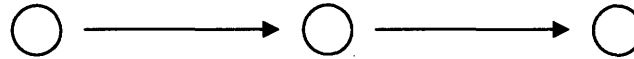
Figure 4.2: Modeling three stations as nodes and the service connecting them as one-way arcs produces a directed graph.
