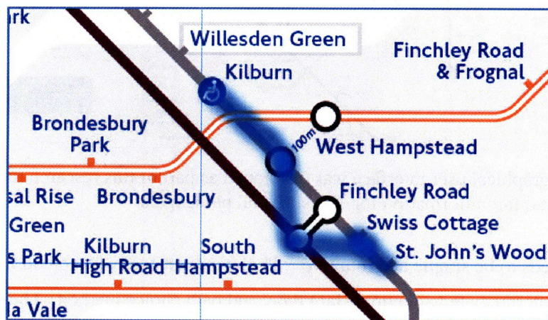
Figure 4.17: The path drawn using default station coordinates is misaligned as it passes through Finchley Road Station because the map represents the same station at different coordinates for the Jubilee and Metropolitan lines.
