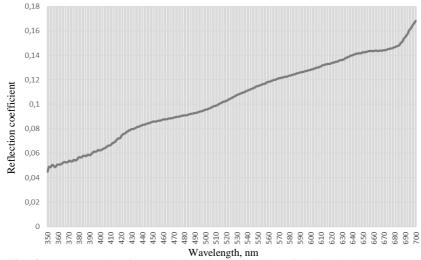
Fig. 2. An example of quantitative determination of soil color by a spectral reflectance curve.
