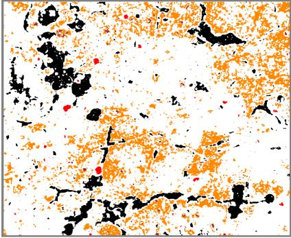
**Fig. 1.** The output of automated analysis of thin section of soil. Color code: black – pores and voids (7.27% of the total area and thin section), red – large mineral grains (0.38%), brown – ferruginous concretions (0.28%), orange – ferruginized areas (15.38%) and white – background (76.68%)
