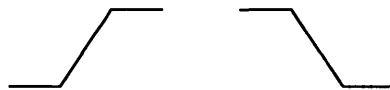
Figure 2-3: These two sections of the hexagonal grid, laid end to end, can be used to approximate any line segment which forms an angle \theta \in [0, \pi/6] with the x -axis.
