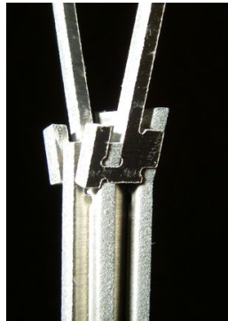
Figure 6. Waterjet cut aluminum mullion.
