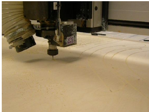
Figure 4. A three-axis Computer Numerical Control (CNC) machine in operation.
