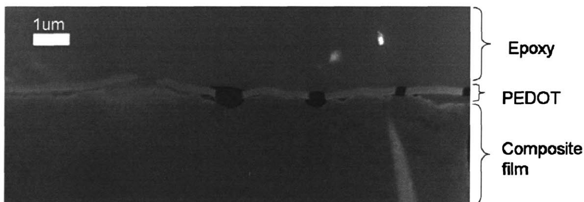
Figure 5-10: Cross-sectional STEM of CVD PEDOT film on POEM- b -PBMA/ \text{VO}_x film.
