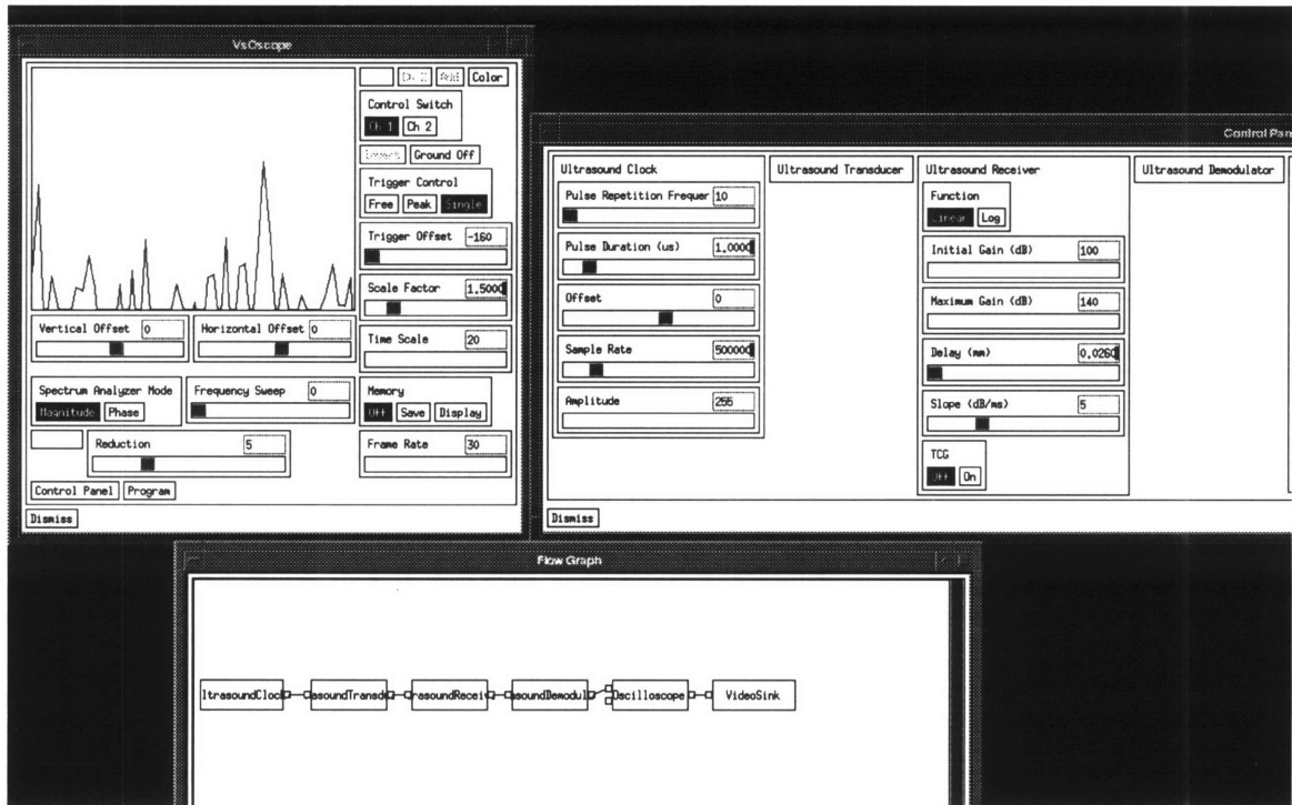
Figure 1-3: The Display, Control, and Program Windows of the Prototype Ultrasound System
