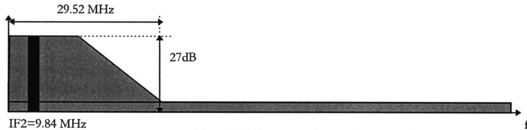
Figure 1.9 Performance requirements for the anti-aliasing filter
