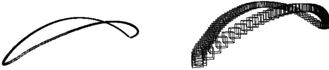
Figure 5-5: The interval curves approximating a set of points on the blade shown in Figure 5-17, with different knot vectors.
