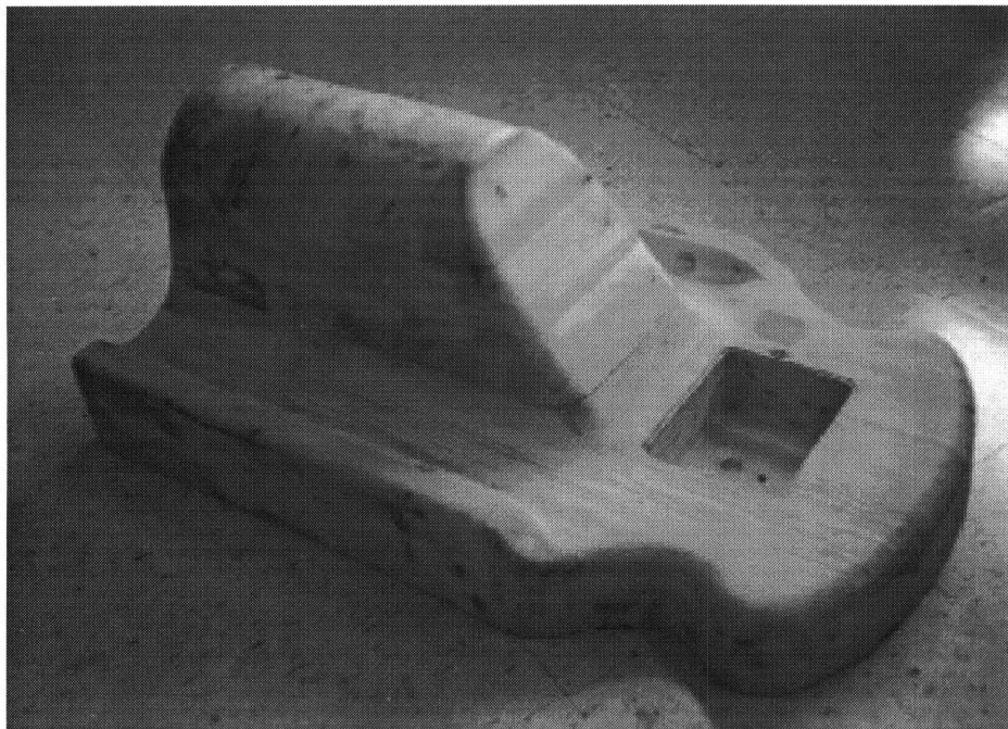
Figure 13: Hydro-Board Completed Bottom Housing Mold
