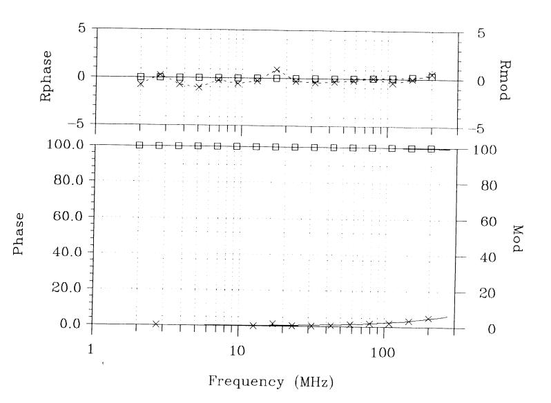
**Figure 8.** Phase (crosses) and modulation (squares) based estimates of the average fluoresescence lifetime at 2- 200 MHz modulation frequencies of filtered coastal seawater irradiated at 406 nm with a KV418 high band-pass emission filter.
