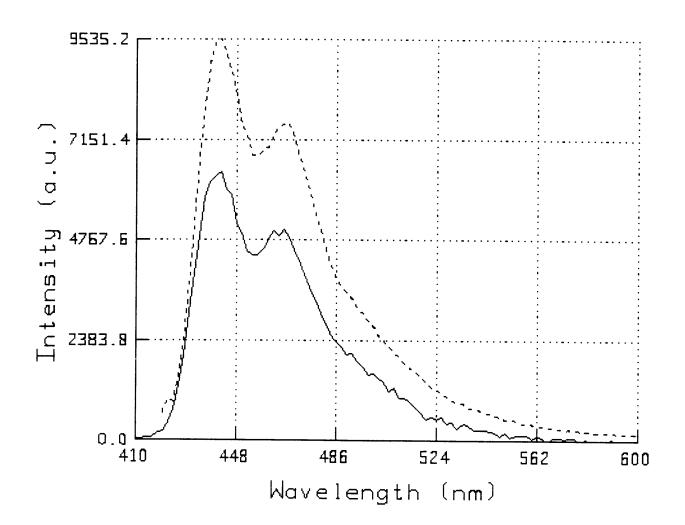
Figure 2. Corrected fluorescence emission spectrum of filtered inner Casco Bay seawater excited at 355 nm.
