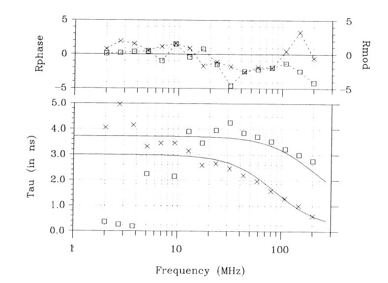
**Figure 7.** Frequency spectrum of phase-shift (crosses) and demodulation factors (squares) of filtered coastal seawater irradiated at 406 nm with a KV418 high band-pass emission filter.
