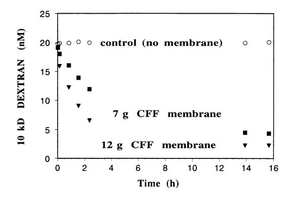
coefficient for DEX between the CFF membrane and seawater was about 100  $L_{sw}/kg_{memb}$ . This would correspond to a  $F_{loss}=0.9$  for the membrane-seawater ratios found in the intact CFF system. Hence, this sorption result can explain the bulk of the losses found for the intact CFF system (Fig. 5).
