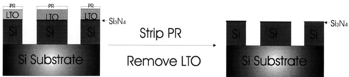
Figure 3.13: Si trenches are finally defined.
