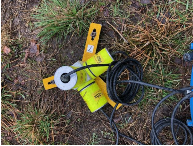
Fig. 2. Acceleration sensors mounted on the ground close to the building.
