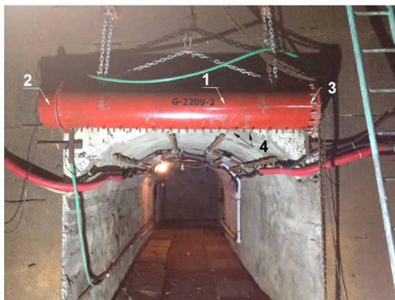
Figure 2. Photo of the absorber in the tunnel of the underground experimental base. 1 –water container, 2 - system activation block, 3 – pyrotechnic device, 4- nozzles
