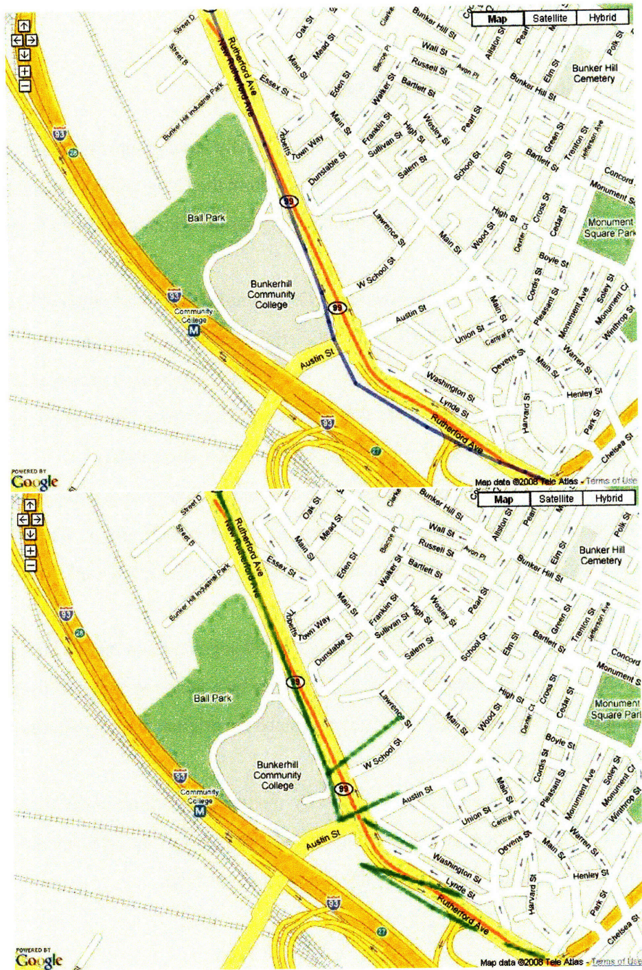
Figure 5-1: Map Matching Result. The red line is actual GPS points reported from the CarTel node and blue line is a sequence of segments that were matched by Algorithm 1 (left). The green line is a sequence of segments that were selected without post-processing (right).
