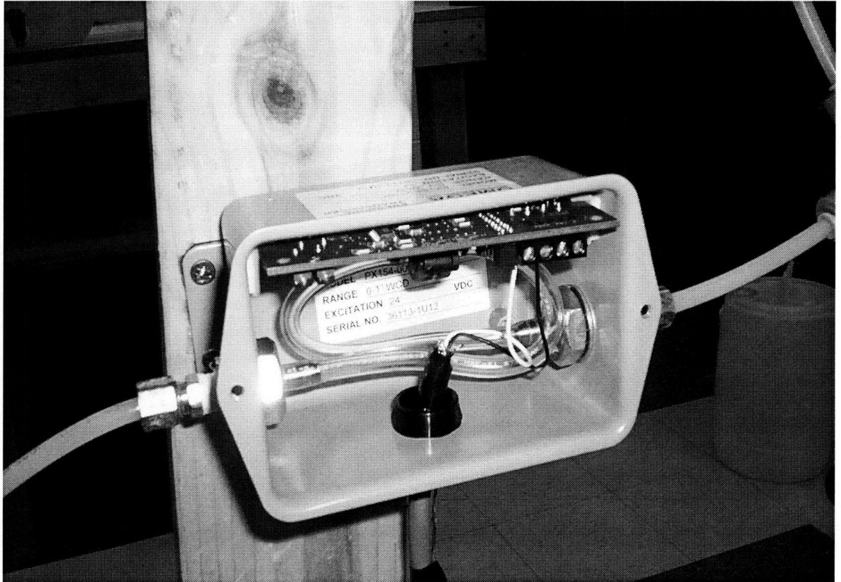
Figure 3.4: Displayed above is the pressure transducer used to measure the pressure drop of the experimental loop
