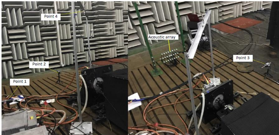
Fig. 3. Four points of far-field microphone test for the electric vehicle motor.
