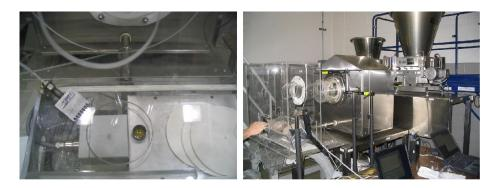
Figure 5-3: NIR Setup on the Zigzag Blender
