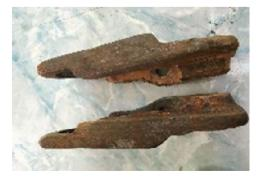
Fig. 1. Wear on chain surface.
