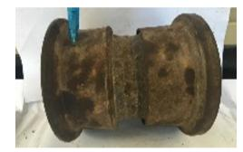
Fig. 3. Wear on surface of roller.
