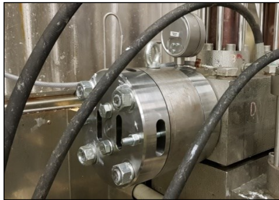
Fig. 6. Detail of the screws assembly built into the high pressure pumping system.
