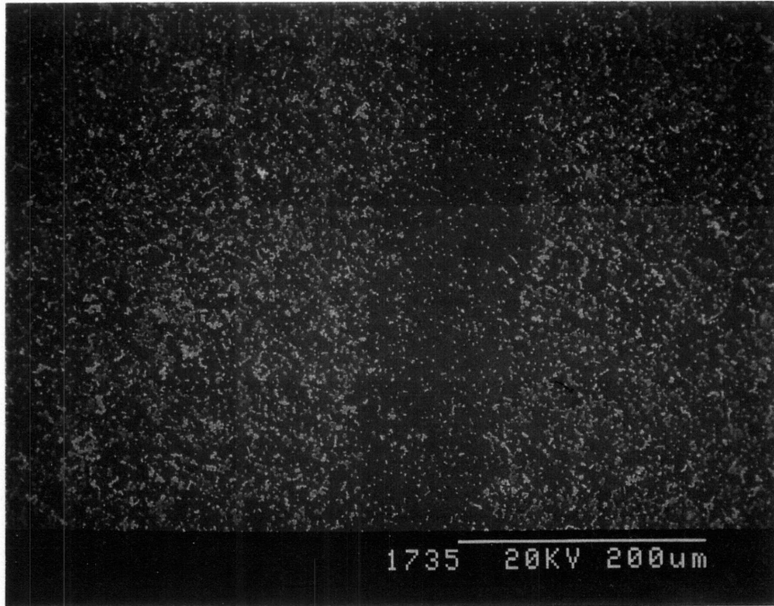
FIGURE 47 : 1.0W AT 3 cm/s; 200x - LINE WIDTH = 110\pm 5\mu\text{m}
