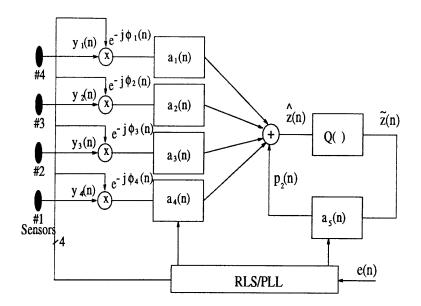
Figure 4-17: The multichannel version of the DFE, running on four data channels. The RLS is jointly adapting all filter coefficients.
