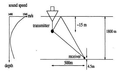
Figure 3-16: The geometry of the Autec experiment. The transmitter is suspended from a boat and the receiver is bottom mounted.
