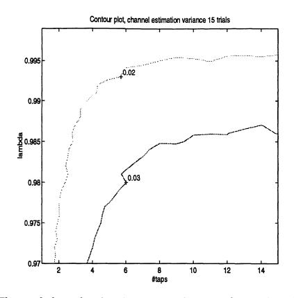
Figure 4-33: The total channel estimation error variance vs the number of taps L and the forgetting factor  $\lambda$  obtained by running the receiver on Doppler spread data. The increase of the variance for low  $\lambda$  and high L is consistent with the theoretical prediction, and it shows the receiver limitation due to ill conditioning of  $\tilde{P}$ .
