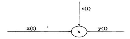
Figure 3-6: A simplified representation of the impact of a rough time varying surface on a ray.
