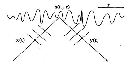
Figure 3-4: Surface Doppler spread, a snapshot of the time-variant rough surface which is modeled as a random process. We use the time-averaged reflection coefficient, therefore only the specular direction is shown
