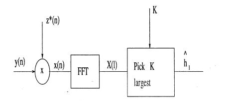
Figure 4-21: The channel tracking of a doubly spread channel implemented with block processing.
