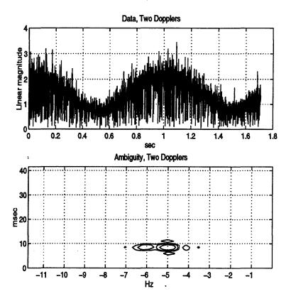
Figure 2-4: The complex envelope (upper panel) and 3 dB contours of the crossambiguity function (lower panel) for a signal with two Dopplers.
