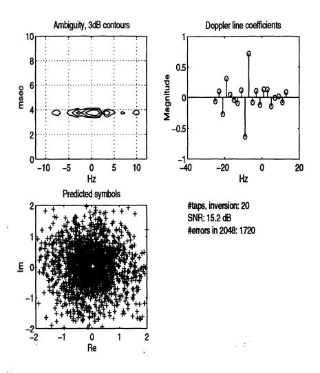
Figure 4-48: Decoding using the FFS Doppler lines and the block channel estimator. The channel response contains a continuous Doppler spread with nearly flat spectrum over its bandwidth.
