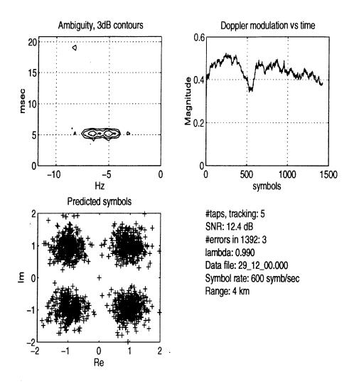
Figure 4-52: Decoding and channel tracking of purely Doppler spread data from the Gould Island experiment. The mean Doppler is from transmitter vessel drift.
