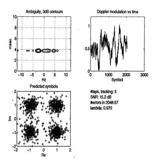
Figure 4-47: Decoding using the IFS Doppler line and recursive channel tracker. The Doppler spread is generated from band limited white noise.
