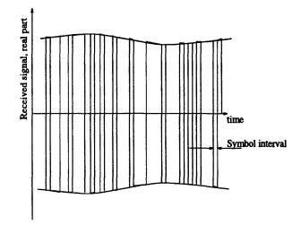
Figure 4-2: The time-variant channel modulates the received signal, but the channel variation is much slower than the symbol rate.
