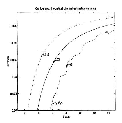
Figure 4-31: The theoretical total channel estimation error variance vs the number of taps L and the forgetting factor  $\lambda$ . The increase of the variance for low  $\lambda$  and high L shows the receiver limitation due to ill conditioning of  $\tilde{P}$ . The Doppler spread is 5 Hz and the SNR is 6 dB.
