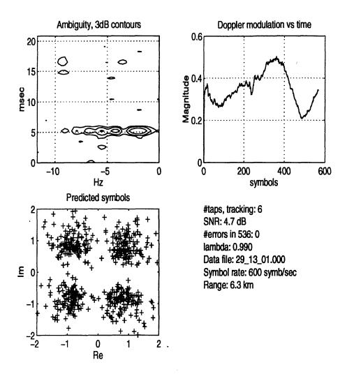
Figure 4-54: The transmitting vessel was drifting, and the received signal level is very sensitive to transmitter depth.
