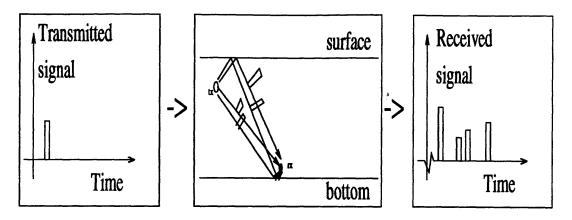
Figure 3-3: The delay structure of the received signal can be derived from the raytrace picture.
