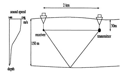
Figure 3-19: The geometry of the Florida experiment. Both transmitter and receiver are suspended from moving boats.
