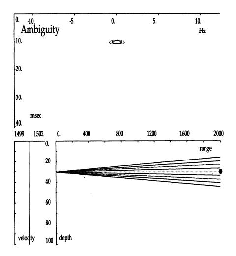
Figure 3-7: Isovelocity example, there is no motion of receiver or transmitter and the vertical beamwidth of the transmitter prevents boundary interaction. The extent of the ambiguity function is given by signal bandwidth and duration.
