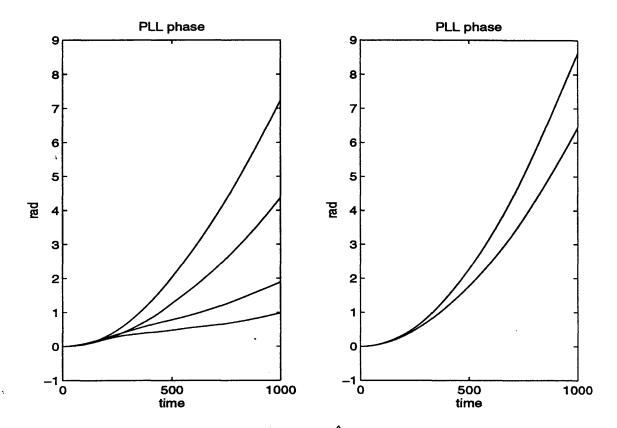
Figure 4-18: The PLL output phase estimate  $\hat{\phi}(n)$  when applied to channels 1-4 (left) and channels 1-2 (right) of real data. The four channels are believed to have the same Doppler because they were recorded from elements closely spaced and mounted on a rigid platform, but the PLL estimates are different. The two channels 1 and 2 are estimated differently when channel 3 and 4 are not used.
