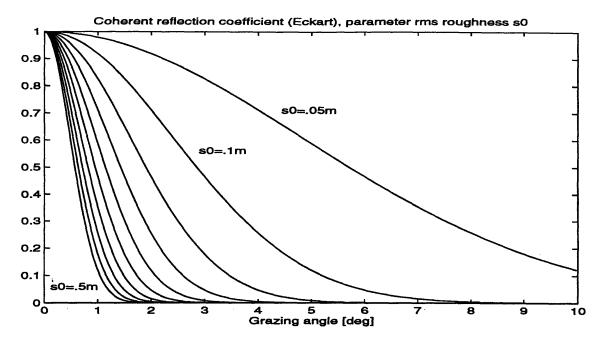
Figure 3-5: Average reflection coefficient vs grazing angle (angle with respect to the horizontal plane). The curves are parameterized by the rms roughness s0 going from 0.05-0.5 m.
