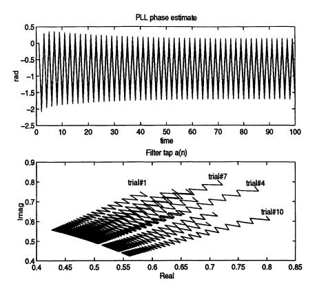
Figure 4-14: 10 trials of the state trajectories when perturbing the filter tap with a small random value  $\delta a$  away from the stationary region. The top picture is PLL phase estimate, and the bottom picture is the complex filter tap values.
