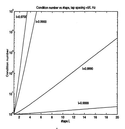
Figure 4-32: The condition number of  $\tilde{P}$  vs the number of taps L for different forgetting factors  $\lambda$  and a Doppler spread of 5 Hz at a symbol rate of 2500 symb/sec.
