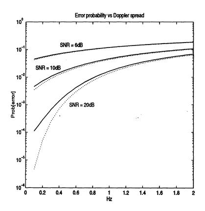
Figure 4-35: The probability of decoding error vs Doppler spread for a doubly spread channel with the SNR as parameter. The symbol rate is assumed to be 600 symb/sec and the delay spread is 5 msec. The dotted lines are the probability of error when the decision errors are not fed back to the channel tracker.
