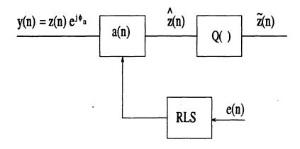
Figure 4-5: The matched receiver that must handle the Doppler shift in the input signal. With no ISI the feedback part of the DFE is absent.
