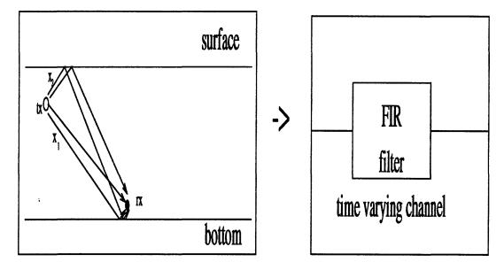
Figure 3-2: Time varying, clustered channel with four taps in the FIR filter.
