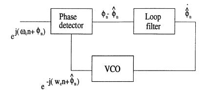
Figure 4-10: Building blocks of a PLL.
