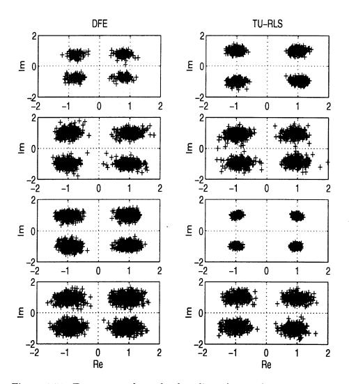
Figure 4-51: Eye pattern from the decoding of some data transmissions in the ocean. The left column shows results obtained with the DFE, and the right column shows results when using the new receiver.
