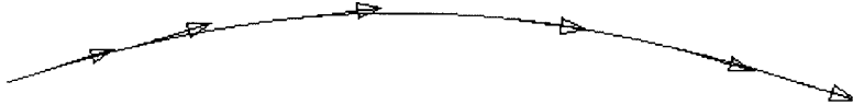
Figure 4-7: Mean camber line designed to generate loading distribution shown in Figure 4-6 with C_l = 1.5 and \epsilon = 5^\circ . Velocity at the node points is also illustrated.
