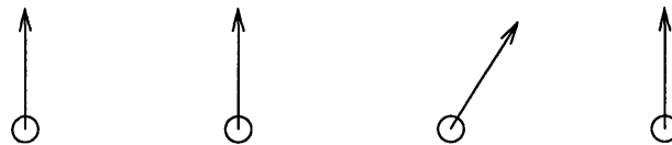
Figure 6-1: Set of data points and prescribed normals to which it is impossible to fit a 4 th order B-spline curve with only 6 control vertices.
