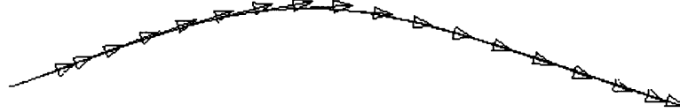
Figure 4-8: Mean camber line designed to generate loading distribution shown in Figure 4-6 with C_l = 1.5 and \epsilon = 3^\circ . Velocity at the node points is also illustrated.
