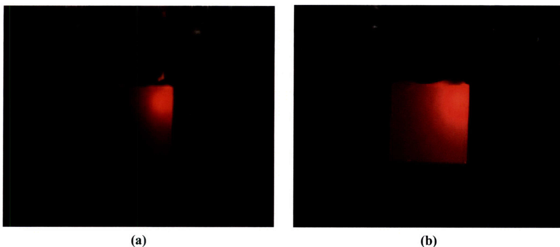
Figure 6-2. Autothermal, steady-state combustion of 40 sccm hydrogen with 2.5 mg of (a) 1wt% Pt on \text{Al}_2\text{O}_3 and (b) 5wt% Pt on \text{Al}_2\text{O}_3 .
