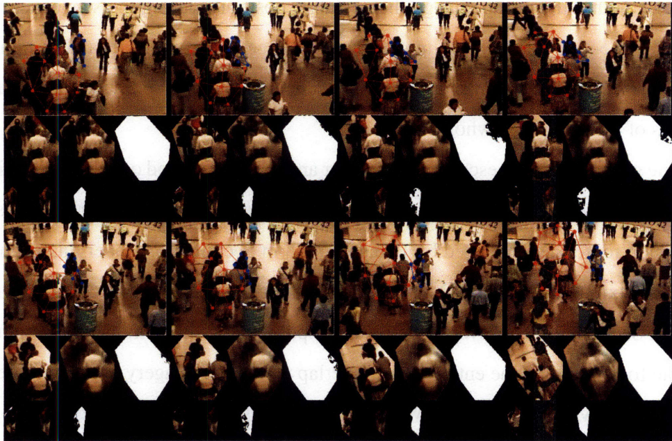
Figure 5-22: Tracking groups of people is more robust than tracking individuals. The blue mesh fails to maintain the track of the individual as she is occluded by another individual within the tracked group. Instead, the mesh continues tracking the occluding figure who then leaves the group. In contrast, the red mesh continues tracking the group successfully through many occlusions and other visual distractions.
