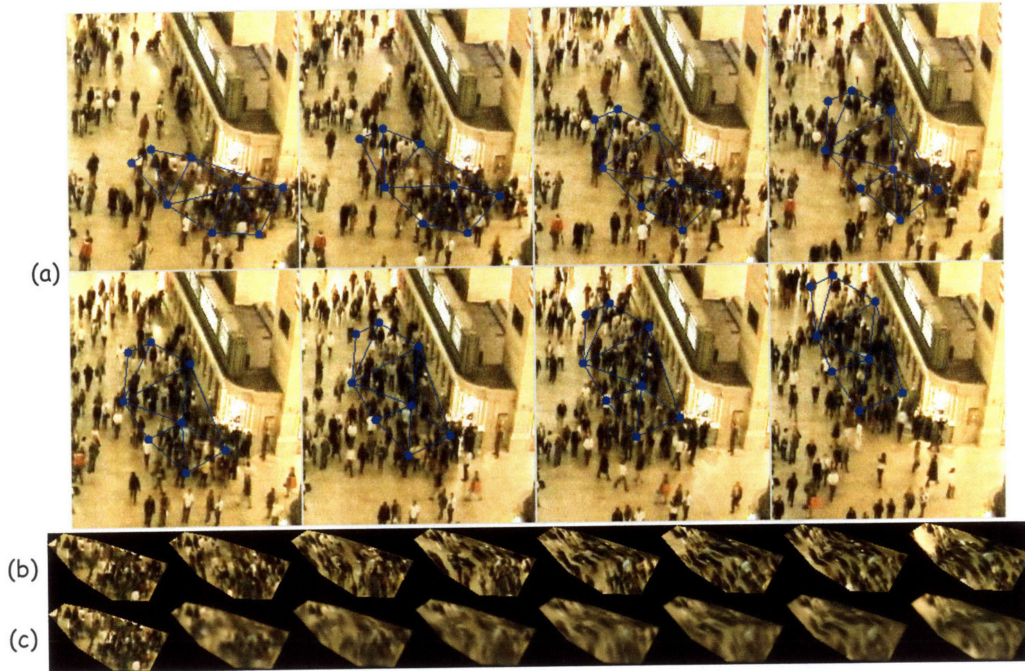
Figure 5-20: Group tracking in densely populated scenes. (a) imagery and detected mesh (b) measurement of shape-free appearance (c) estimated shape-free appearance model
