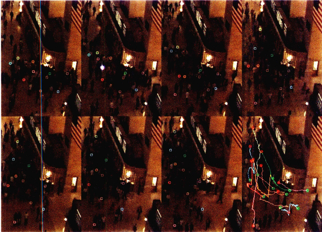
Figure 5-19: Flow-based tracking fails in such dense and busy indoor environments. Constant occlusions and other visual distractions easily confuse local feature trackers. Only two of the original ten points were tracked successfully through the entire sequence. The last frame shows an overlay of the resultant tracks, with circles in green indicating the start of each track and the red circles indicating the end.
