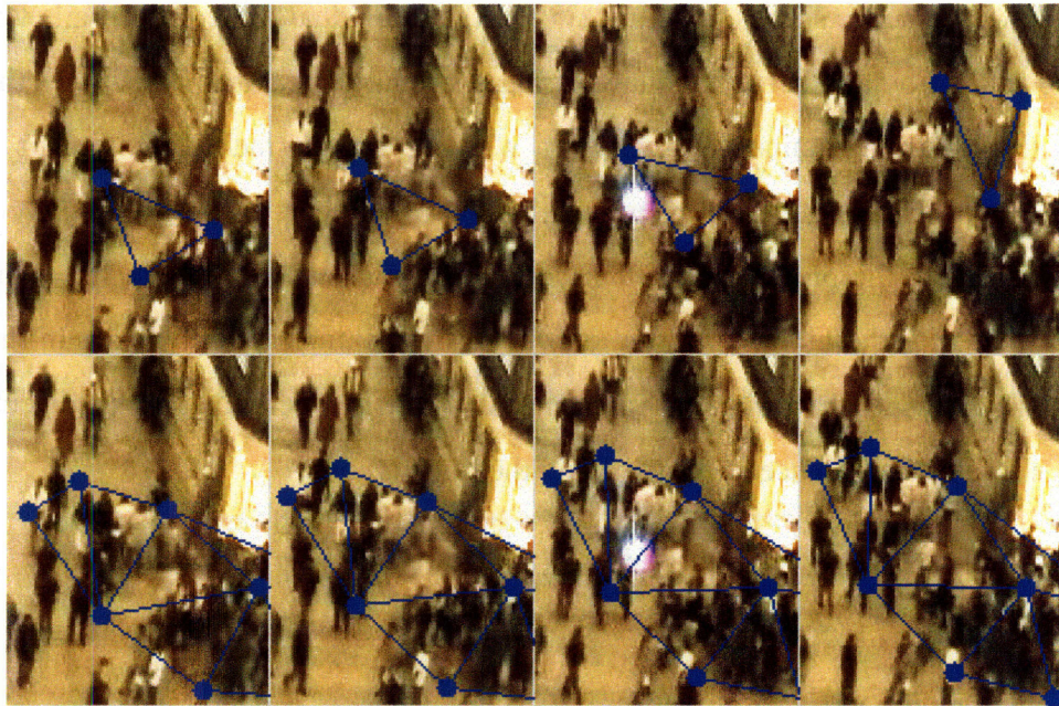
Figure 5-21: Piecewise affine meshes are more robust to error and local misregistrations than are simple affine patches. Top row: the tracked affine patch loses its target in the presence of the camera flash. Bottom: the piecewise affine mesh is robust to the camera flash due to the fidelity of matches elsewhere.
